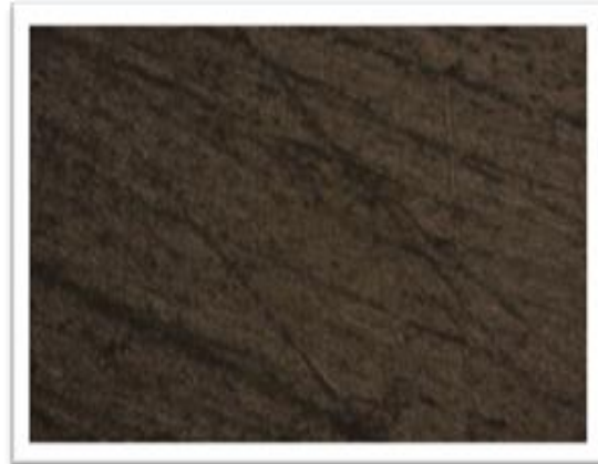
Plate XV: Aluminium 9.37 Copper alloy over aged at 500°C (Caustic etch) x 200°C
