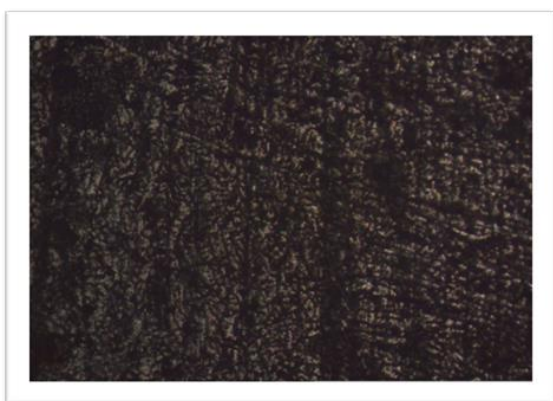
Plate X: Aluminum 9.37 Copper alloy as Cast 350°C for 1 hr. Polarized light, recrystallized grains and bands of unrecrystallized grains (caustic etch)
